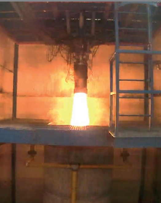
Picture of the first full-power test of PLD Space's liquid-fuel reusable rocket engine.
